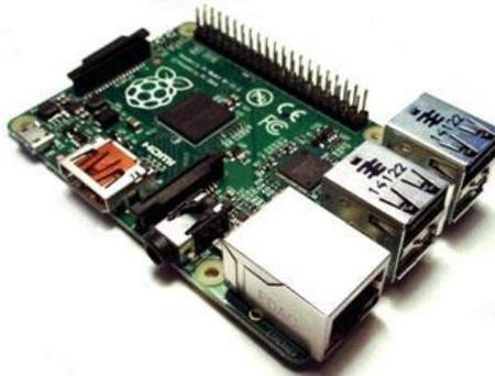
**Gambar 2.6** Raspberry Pi Model B+
