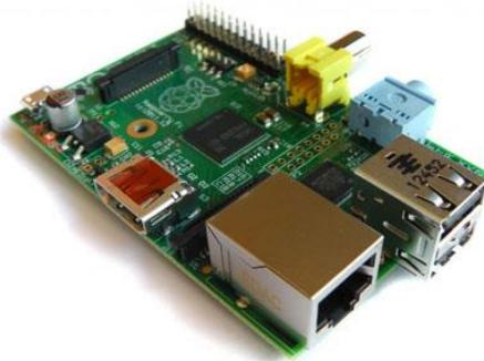
**Gambar 2.5** Raspberry Pi Model B
