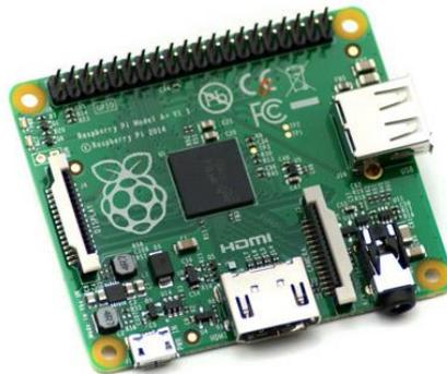
**Gambar 2.4** Raspberry Pi Model A+
