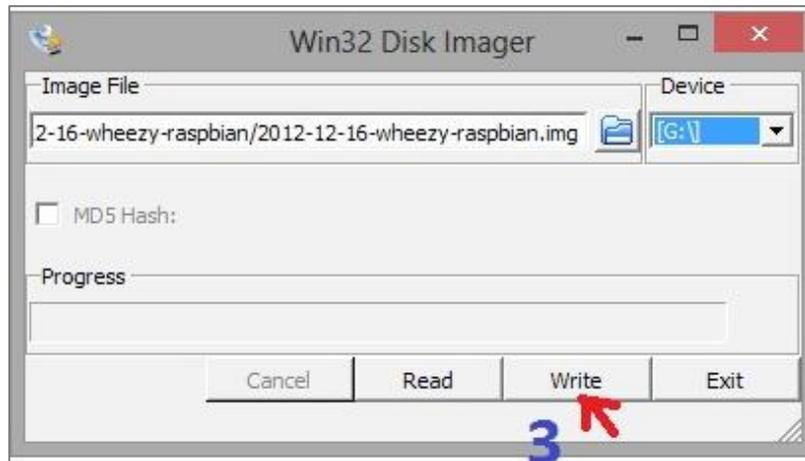
**Gambar 2.9** Write OS Raspbian ke MicroSD Card
