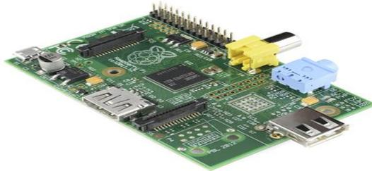
**Gambar 2.3** Raspberry Pi Model A
